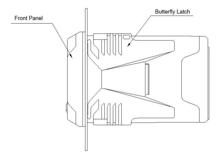
Fig. 3 Schematic diagram of controller disk mounting method
